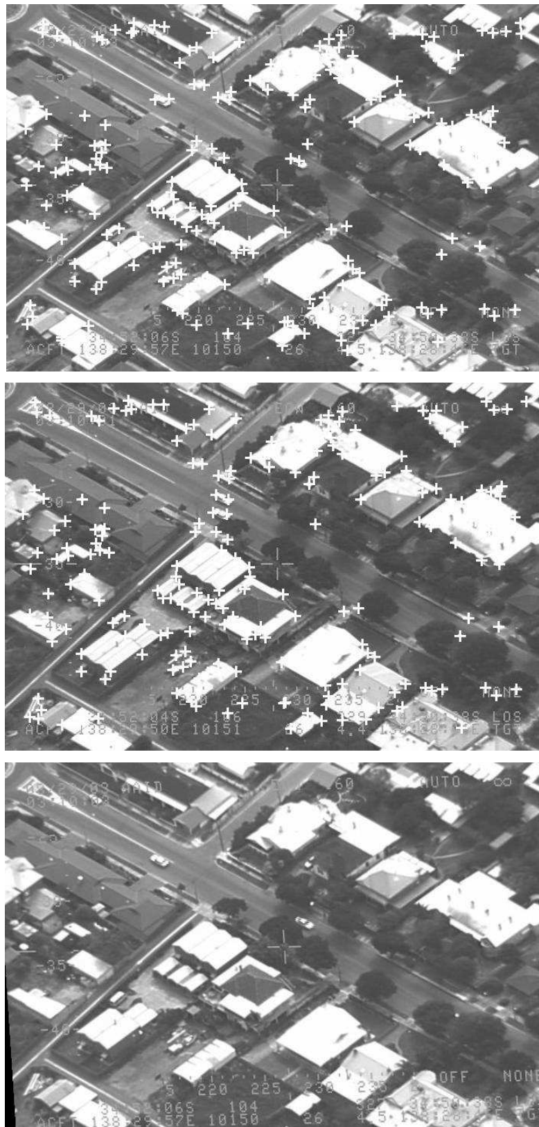
Figure 2: Feature tracking for video registration. Top and middle: two frames from the sequence. Bottom: Top frame registered to the middle frame using affine model fitting to the tracked features.
