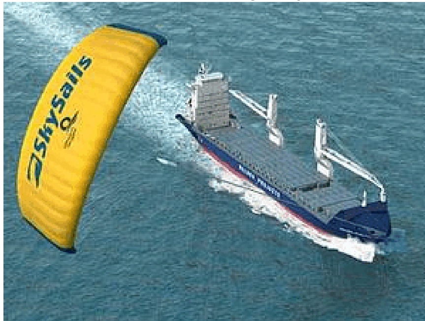
Figure 9. SkySails Concept Applied to Commercial Cargo Ship
