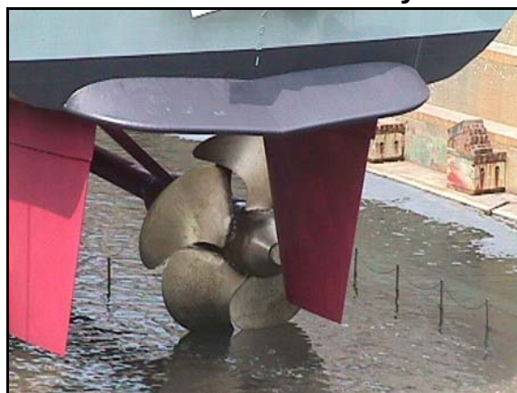
Figure 3. Stern Flap on DDG-51 Class Destroyer
