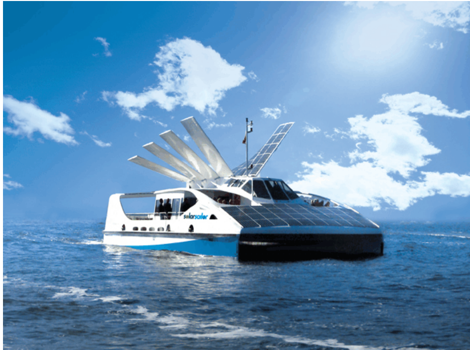
Figure 11. Solar Sailor Hybrid-Powered Ferry Boat
