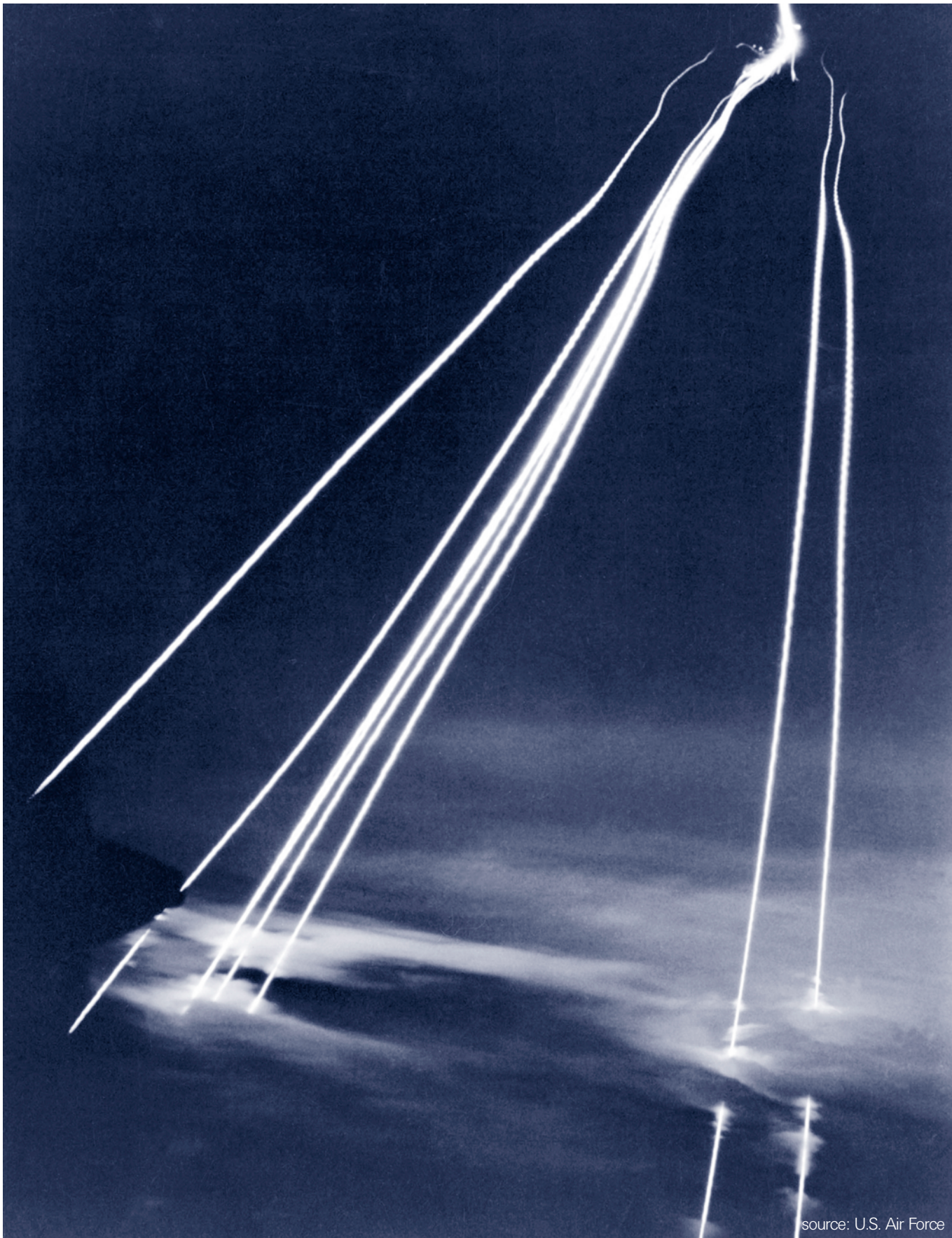
A time exposure of eight Peacekeeper (LGM-118A) intercontinental ballistic missile reentry vehicles passing through clouds during a flight test.
