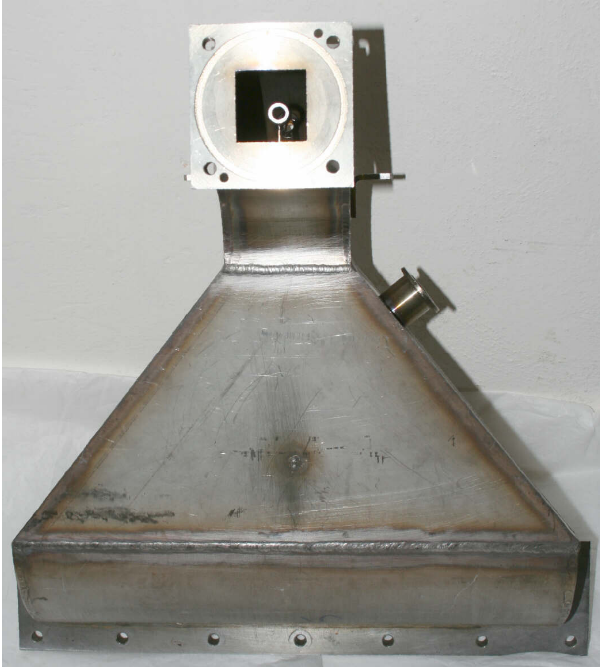
Fig. 15. Photo of the delta input element of the vapor trap
