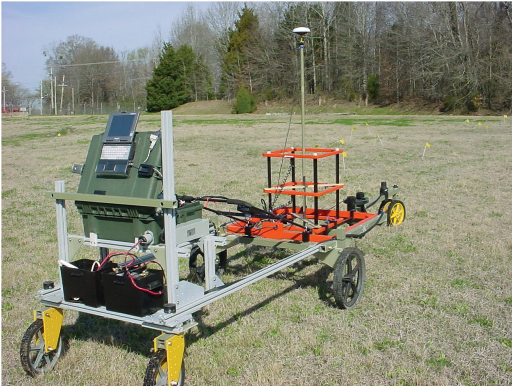
Figure 3. MSS on the calibration lane at the UXO test site.
