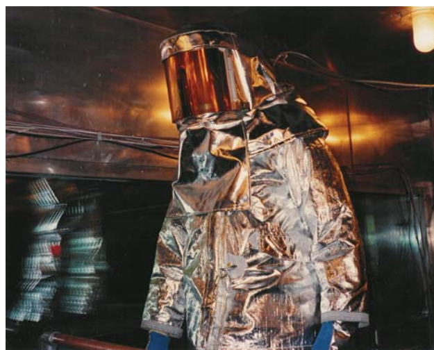
Fig. 19-5. The climate chambers are an important resource in the development of clothing or protective equipment. This 1990 photo shows a firefighting suit developed by the Navy. Although the soldier who is volunteering to test this suit for the US Navy may not derive any direct benefit from his participation in research, this work will benefit thousands of other soldiers, and is thus permissible under the principle of justice . Photograph: Courtesy of US Army Research Institute of Environmental Medicine, Natick, Massachusetts.
