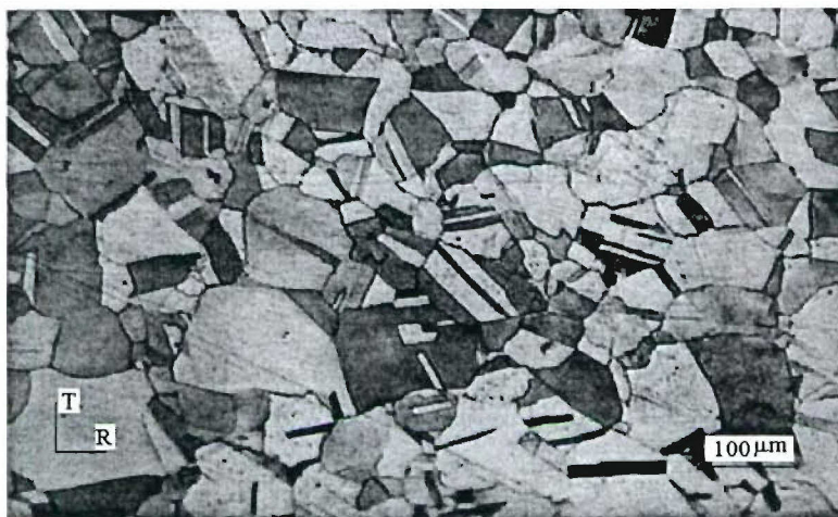
Figure 2.3: Optical micrograph of the base AL6XN stainless steel.
