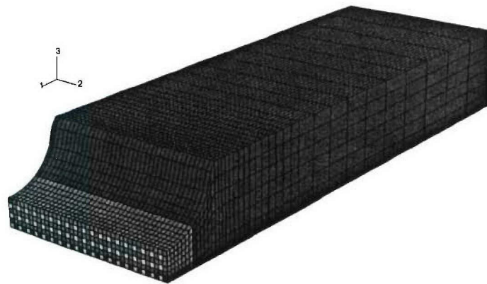
Figure 4.4: Finite element discretization and location of primary nucleation centers for h = 0.5D_v = 66\mu m .
