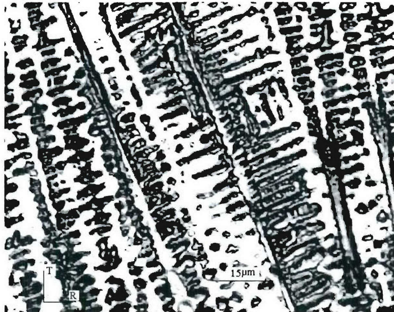
Figure 2.4: Optical micrograph of the weld Inconel-625 superalloy.
