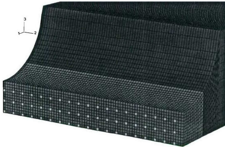
Figure 4.6: Finite element discretization and location of primary nucleation centers. h = 0.25D_v = 33\mu m .
