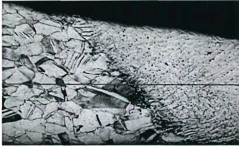
Figure 2.25: Base Material/Weld interface region in AL6XN stainless steel welded plate P_C .
