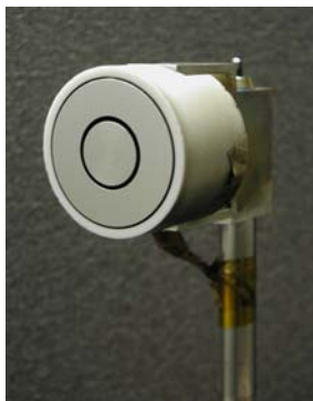
Figure 2. Nude Faraday Cup. Inner collector and sheath seen in above picture with slight gap between.
