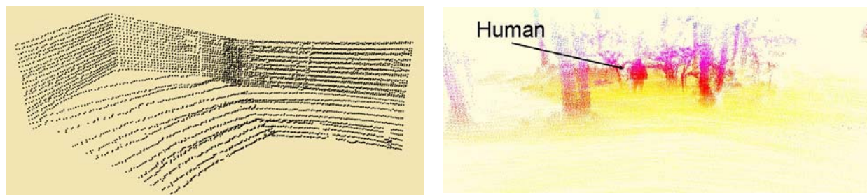
Figure 2. Left figure is a single scan of intersection of two walls at ~15 m; right figure shows several hundred scans of a human in woods at ~15 m, colored by elevation.
