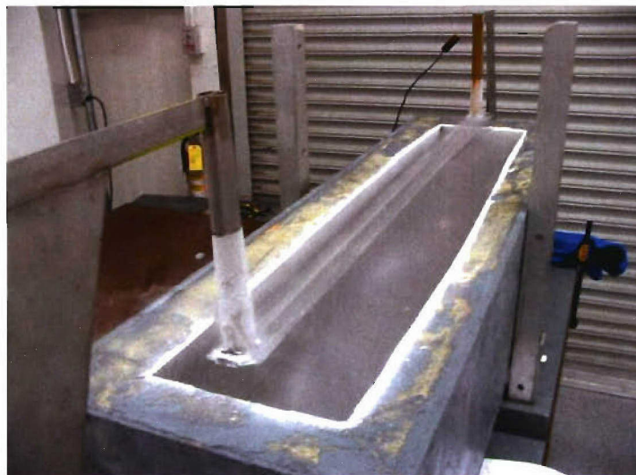
Fig. 7-18. Integrated thermal contraction test rig
