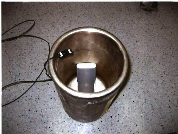
Fig. 5-9. Capacitor pad with inserted thermocouple for cooldown measurements
