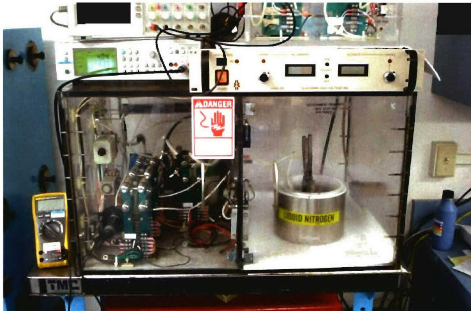
Fig. 6-17. Stamp capacitor test setup with dewar for cryogenic testing
