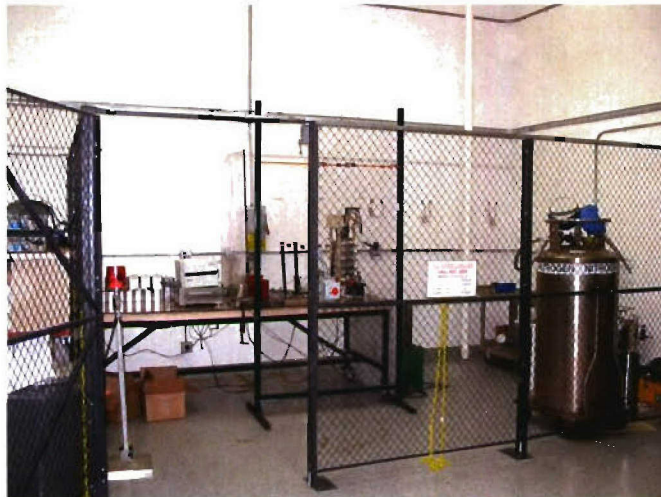
Fig. 6-1. The capacitor test facility at GA. The control and monitoring are located just outside the left edge of the photograph
