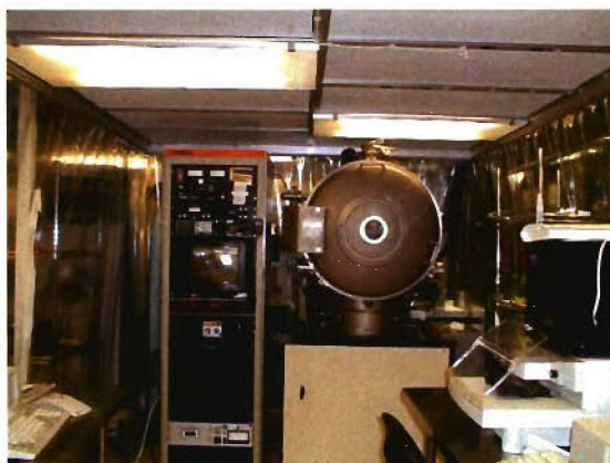
Fig. 6-21. Albany NanoTech's metal evaporation equipment, which can deposit metallization thickness between 20 Å and 5 \mu\text{m}
