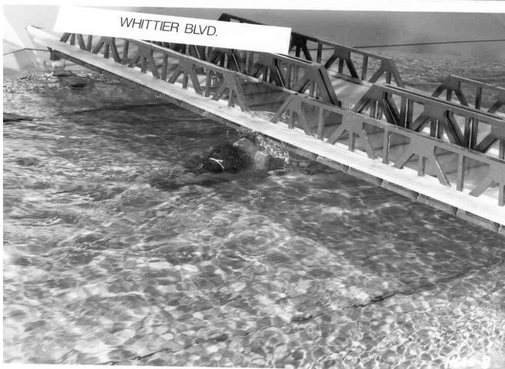
Figure 15. Flow conditions in 1:50-scale model of Rio Hondo River, debris on bridge pier.
