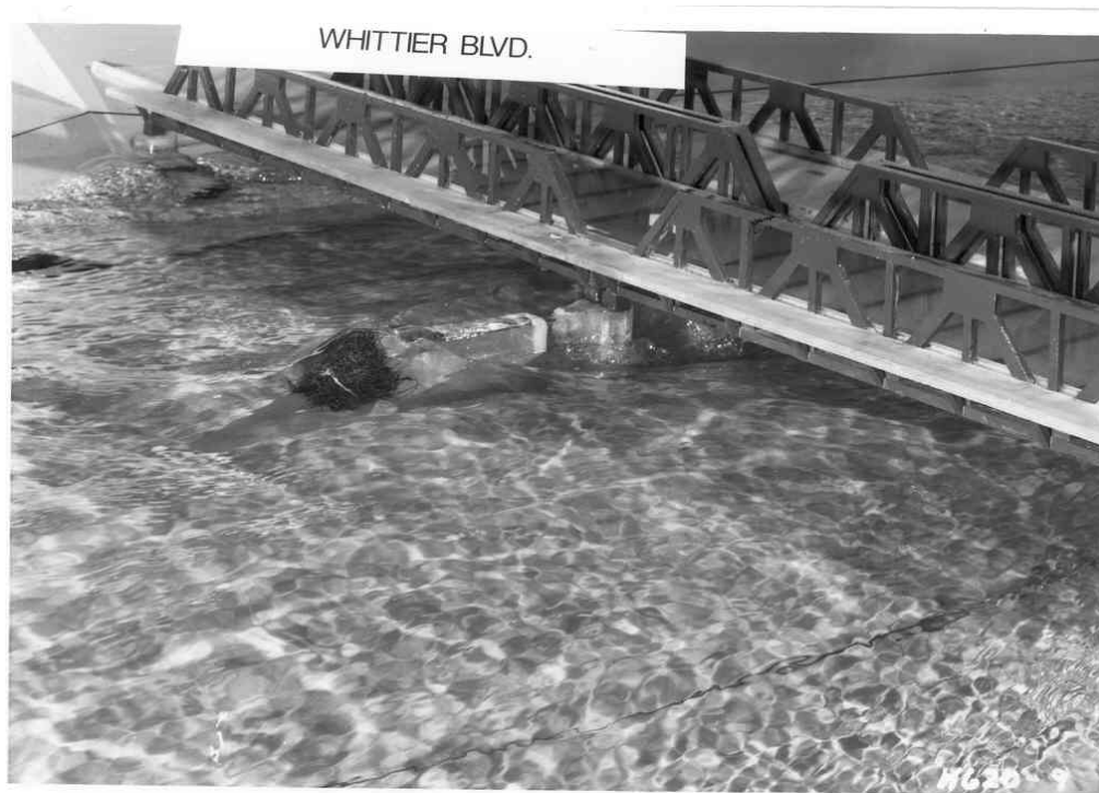
Figure 16. Flow conditions in 1:50-scale model of Rio Hondo River, debris on extended bridge pier.
