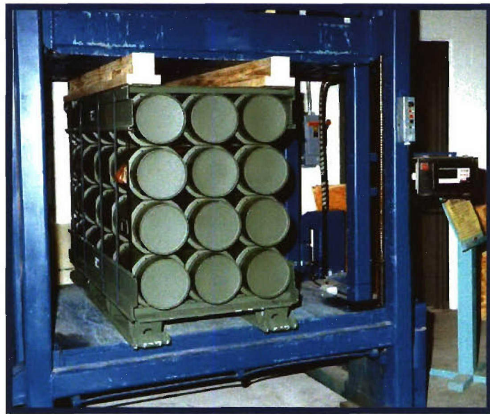
Photo 1. Example of Stacking Test.
