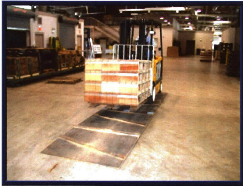
Photo 10. Test Unit Being Carried Over Forklift Course
