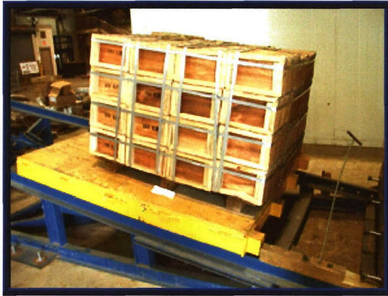
Photo 9. Incline-Impact Testing of the Test Unit.
