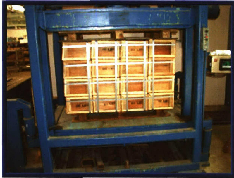
Photo 6. Test Unit in the Stacking Test.
