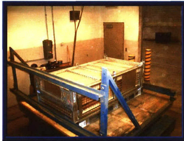
Photo 2. Example of the Repetitive Shock Test. (MSTF Low)
