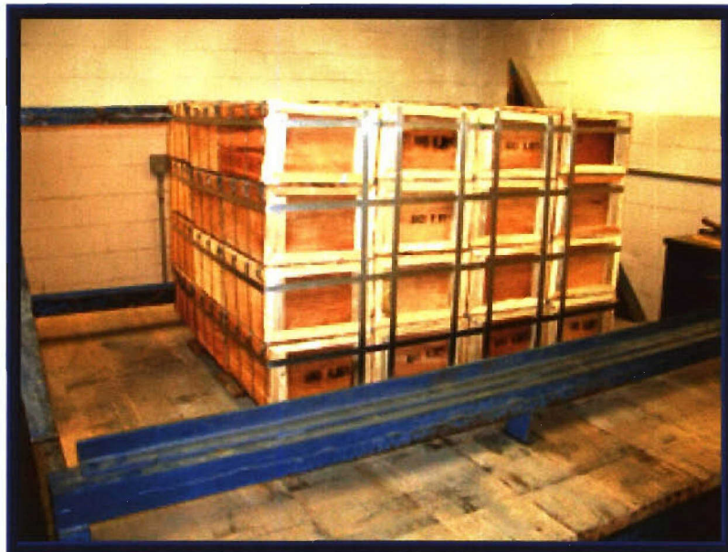
Photo 7. Test Unit During Repetitive Shock Testing.
