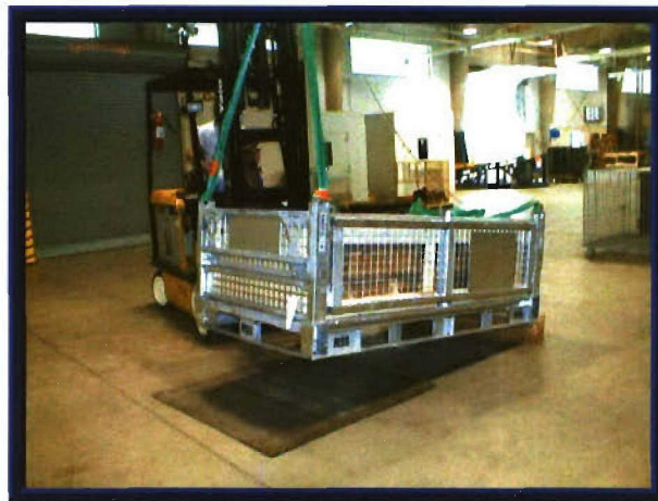
Photo 3. Example of Edgewise-Rotational Drop Test (MSTF Low)
