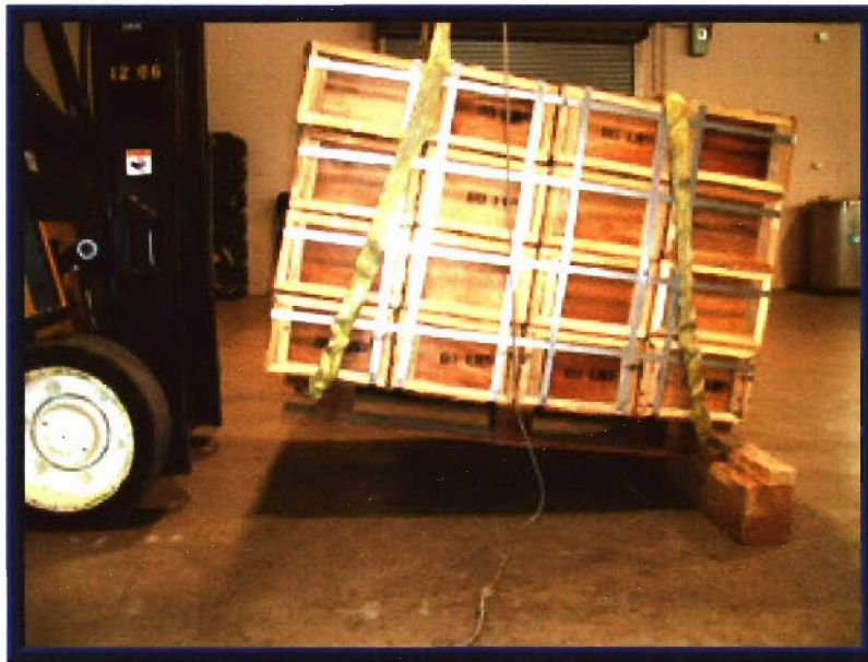
Photo 8. Edgewise Drop Test on the Test Unit.
