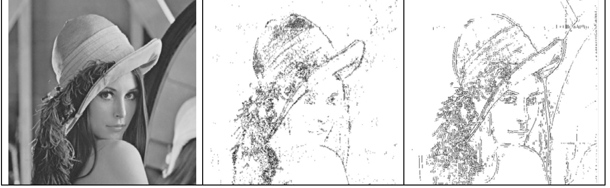
Fig. 1.9 Source image “Lena”; the result of 190-harmonic Fourier-based edge detection method application; and the result of 190 Hermite functions based edge detection method application.
