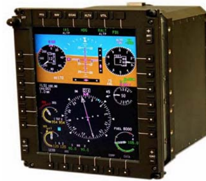
Figure 11. Rockwell Collins MFD-268P
