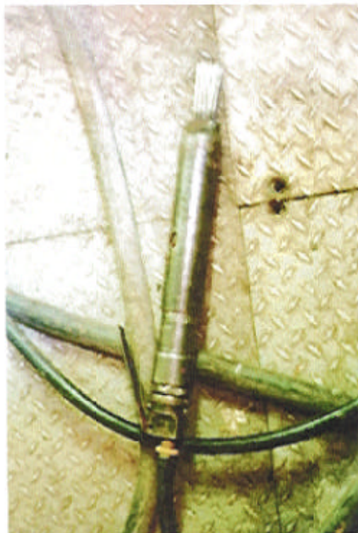
Figure 15: Needle gun used during SATR operations.
