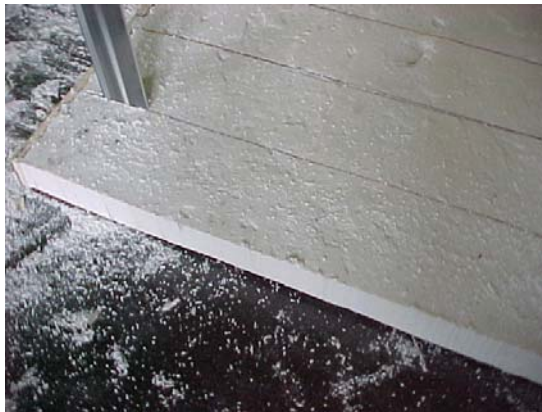
Fig. 6 Cutting beam specimens
