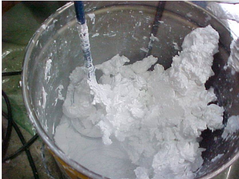
Fig. 2 Mixing rubber latex with microballoons (near the end of the mixing process)
