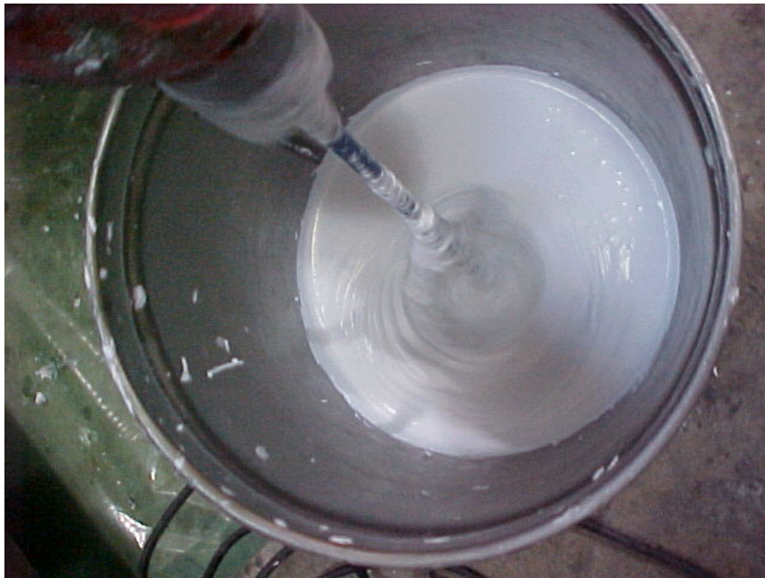
Fig. 1 Mixing rubber latex and microballoons (at the very beginning of the mixing process)
