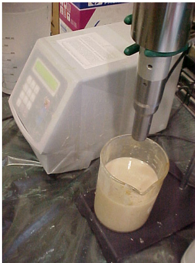
Fig. 3 Mixing nanoclay using the ultrasound mixer
