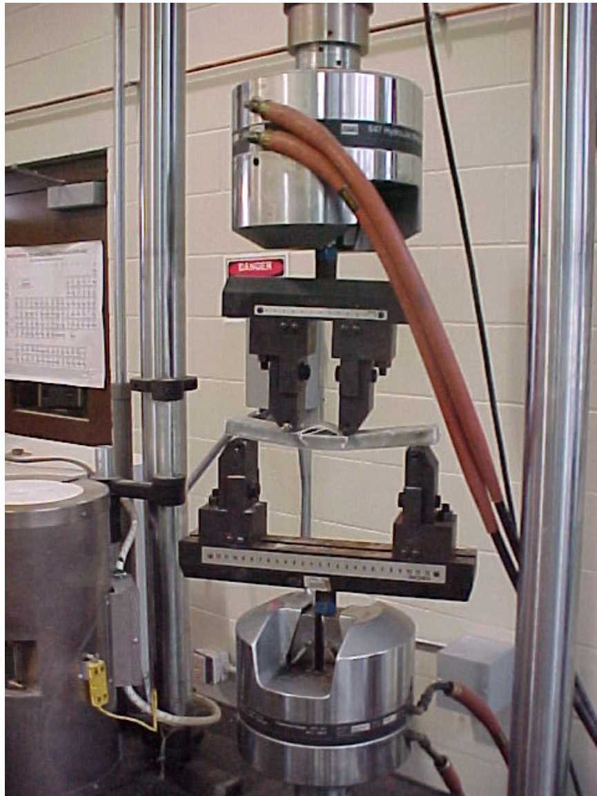
Fig. 9 A sandwich specimen under four-point bending test
