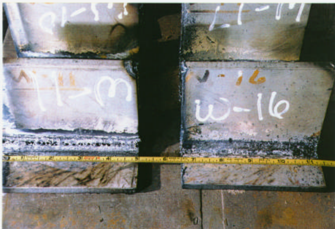
Photograph showing linear porosity along the fusion centerlines of panels W11 and W16 (see Table 3-3, Carboline 8101 and Nippe Ceramo).
