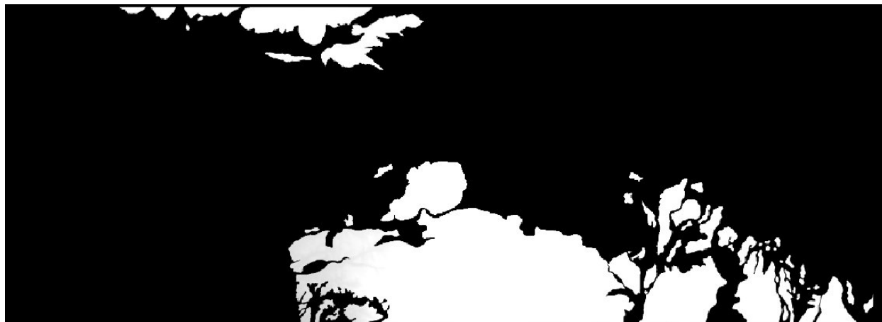
Figure 21. Raster mask created by clipping the original 5-m DEM with the basalt and sedimentary rock landform polygons.
