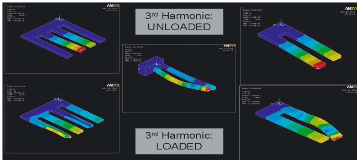
Figure 2. Finite element simulations of the nanomechanical properties of the nanoscale tuning forks. The color indicates the distribution of the strain field in a the dominant normal mode.
