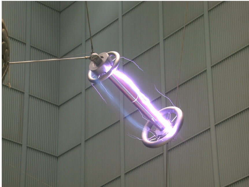
Figure 2. Cutler safety core test at Hydro Quebec.
