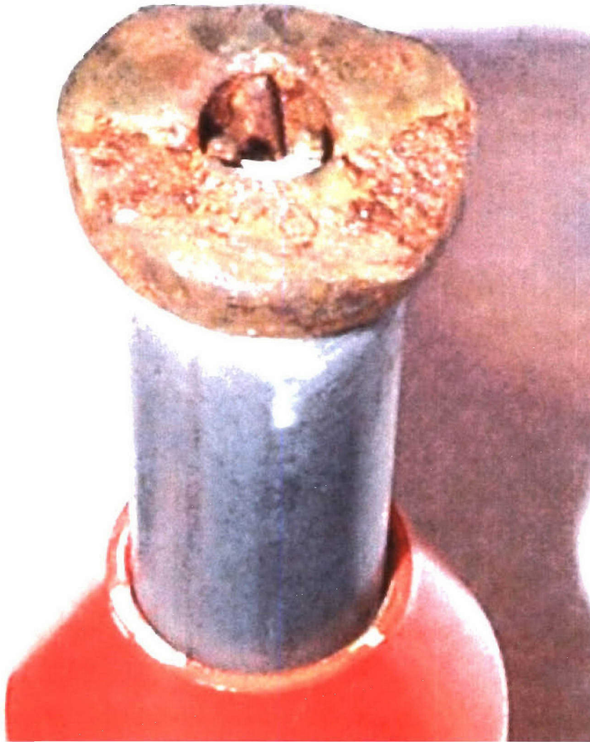
Photograph showing the fracture surface from the returned 1/2 inch swage socket.
