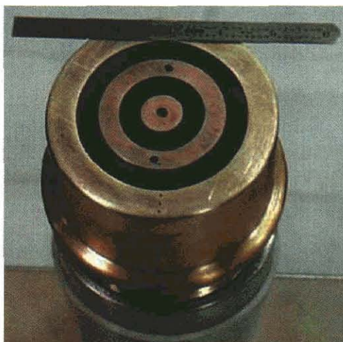
Figure 3-1. Photograph of the shell-on-shell gas nozzle. The inner and outer radii of the outer nozzle exit are 3 and 4 cm; the inner nozzle exit radii are 1 and 2 cm.
