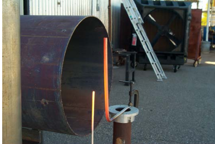
Figure 7. Controlled heat flux combustor operating at 1400 degrees C.
