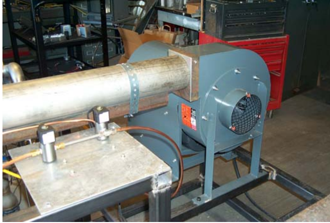
Figure 4. Controlled heat flux combustor blower fan
