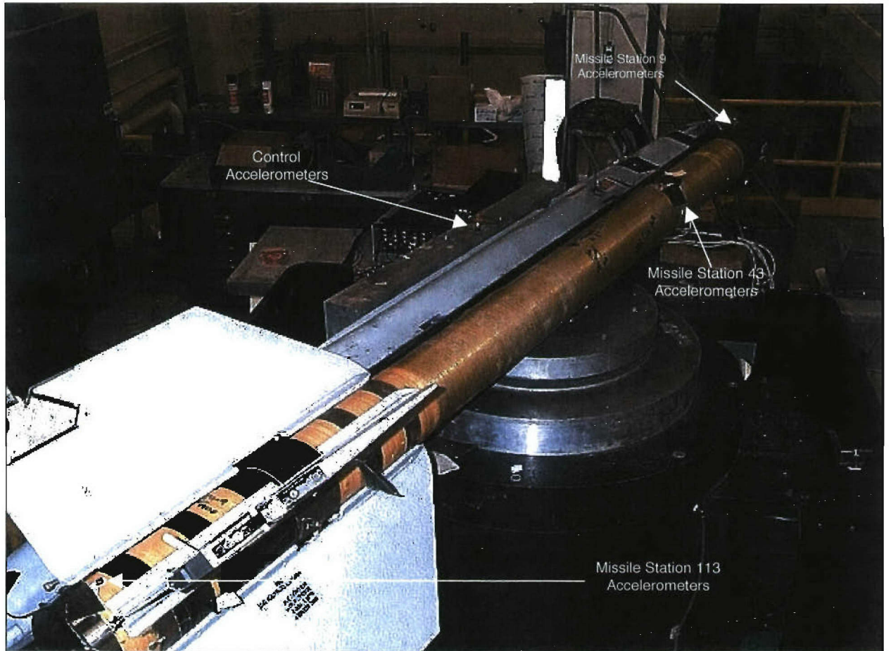
FIGURE R-3. Accelerometer Placement.
