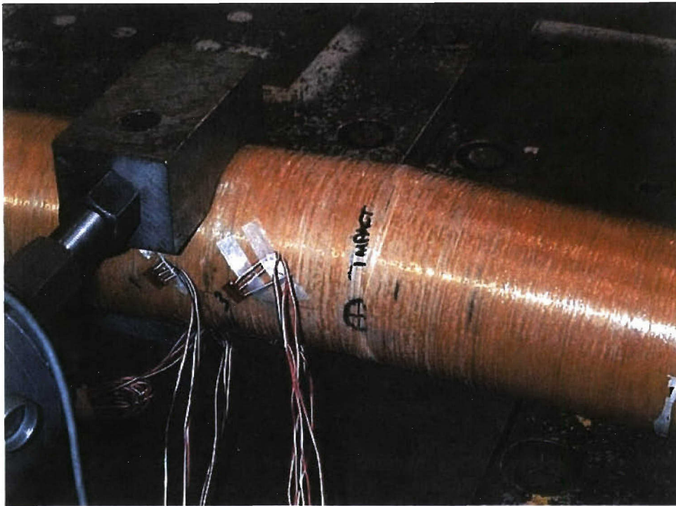
FIGURE T-19. Failed Area of Blue Tube Serial Number 008.
