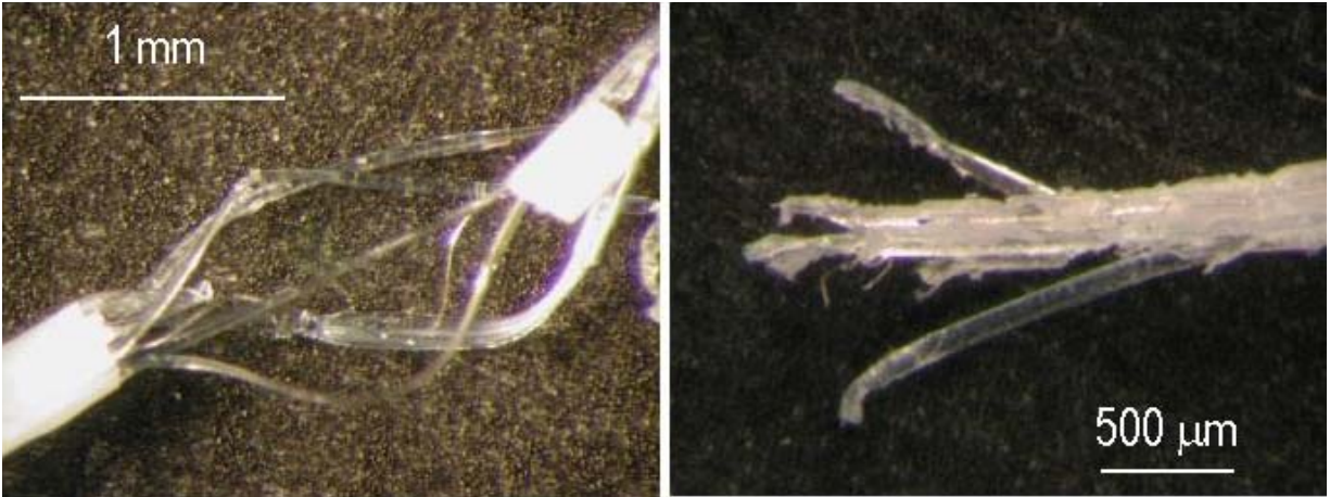
Figure 66. Optical stereo-microscopy image of multilumen preceramic silicone resin microtubes (H44, Filler #2, no coloring agent)
