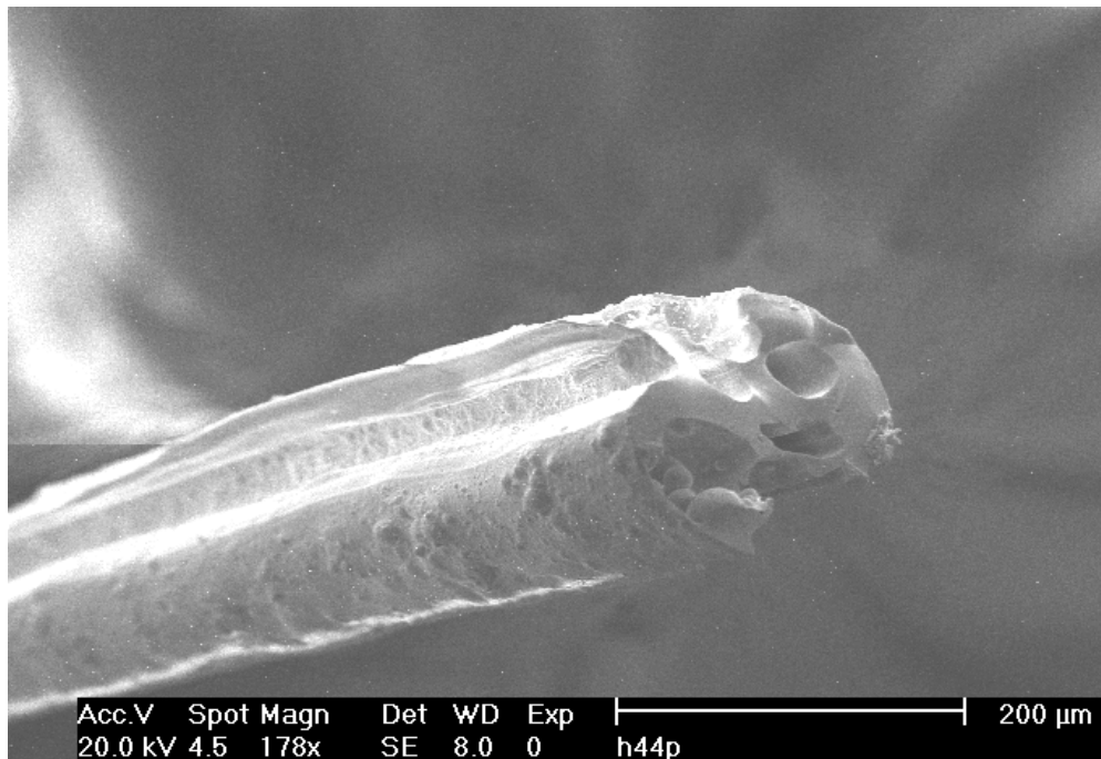
Figure 94. SEM image of a co-extruded multi-lumen microtube, after pyrolysis (H44 and filler #2)
