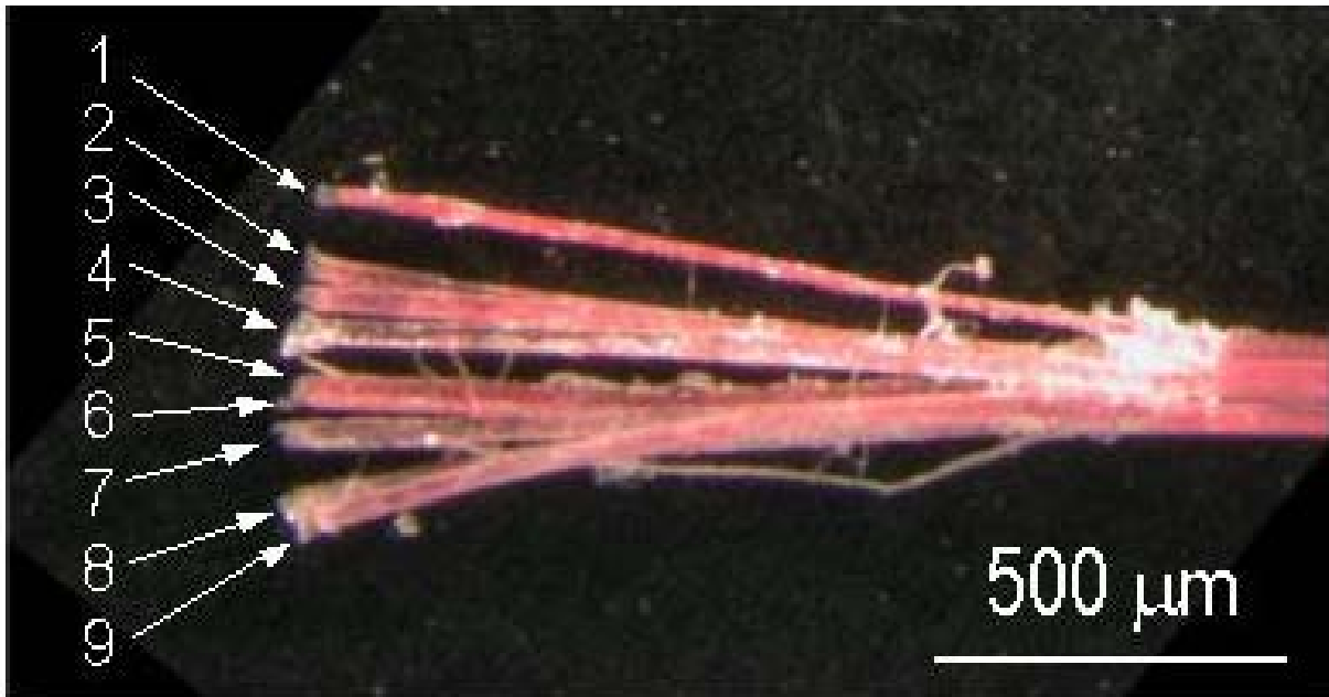
Figure 61. Optical stereo-microscopy image of a multilumen preceramic silicone resin microtube (SOC-A35, Filler #2, red coloring agent)
