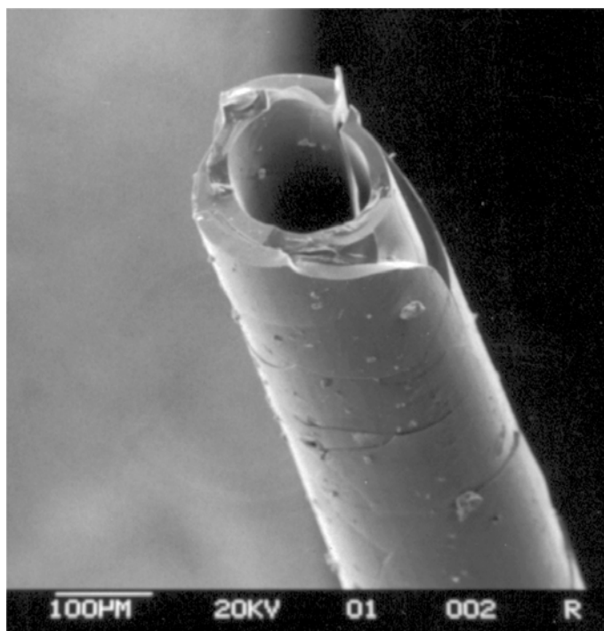
Figure 28. SEM image of a co-extruded microtube not well cross-linked, after pyrolysis (SOC-A35 and filler #2)
