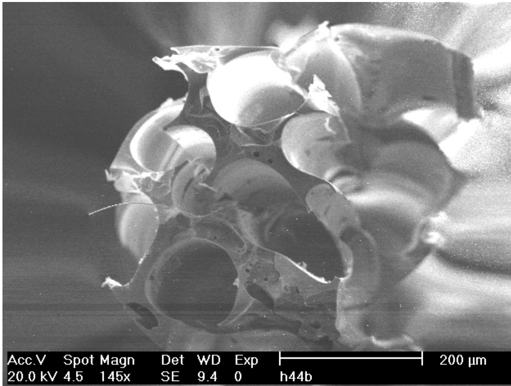
Figure 93. SEM image of a co-extruded multi-lumen microtube, after pyrolysis (H44 and filler #2)
