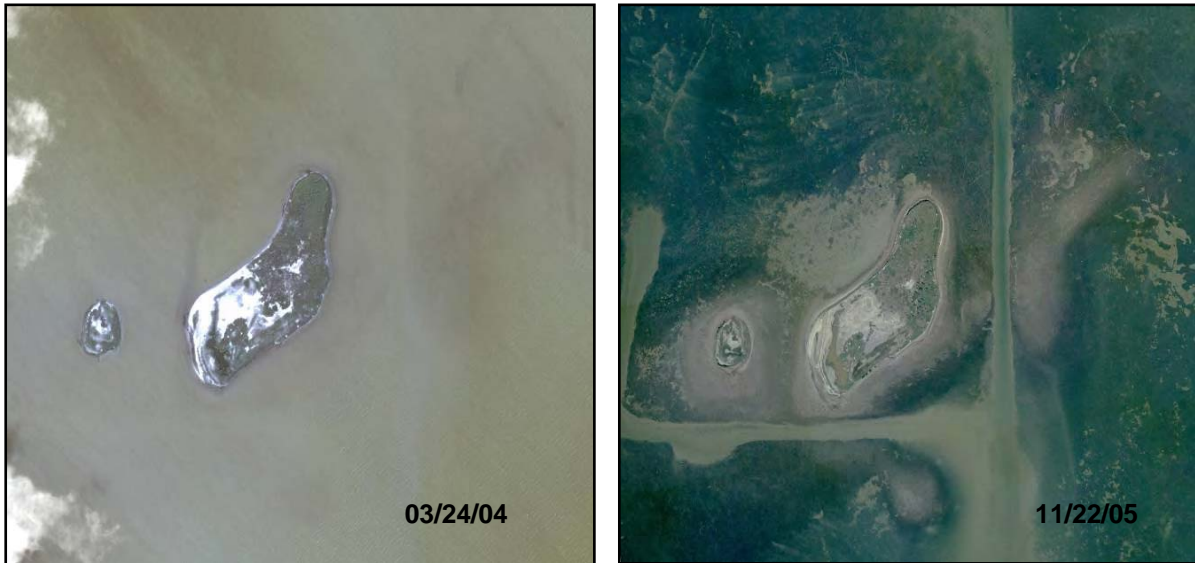
Figure 3. Image on left depicts poor conditions (clouds, high sediment load, and high winds). Image on right illustrates near optimal conditions (acquisition date appears at lower right in each image)
