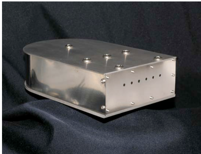
Figure 4. The msLPT is about to undergo final acceptance tests. Six diode lasers drive a special ablation fuel tape behind the output ports. These are fired in matched pairs to maintain a fixed center of thrust. A ns-pulse version is being developed.
