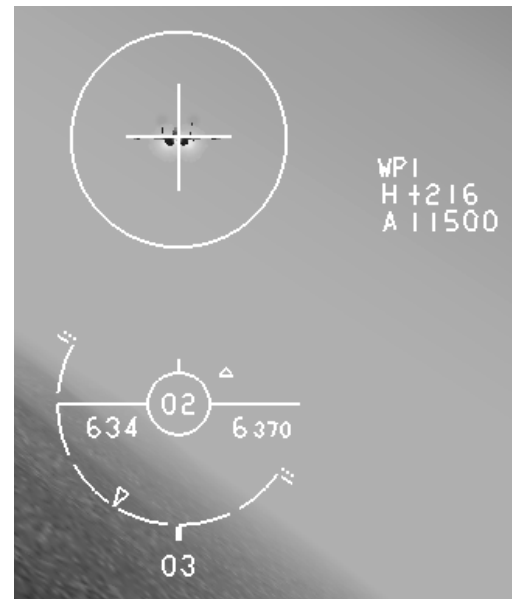
Figure 6: NDFR Display. In this figure, the simulated aircraft is rolled left 30°, pitched up 2°, with an airspeed of 634 knots, an altitude of 6,370 ft, and heading north at 3°.
