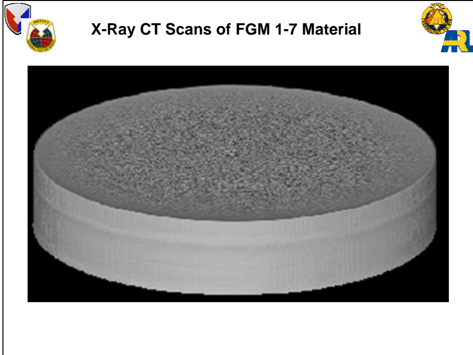
Figure 7. X-ray CT scans of FGM 1–7 material.
