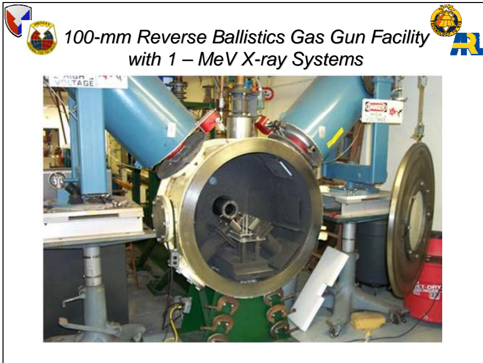
Figure 20. The 100-mm reverse ballistics gas gun facility with 1-MeV x-ray systems.
