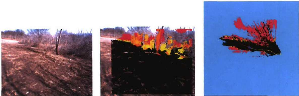
Figure 11. Terrain Perception: The right image shows raw color data. The middle figure is the same image with masking to show areas of obstacles as classified with the fuzzy logic traversability classifier. The right image is the data projected into a 2 dimensional Cartesian grid that uses magenta to mark dangerous obstacles.
