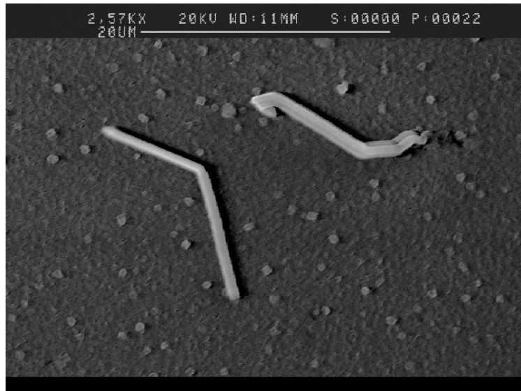
Figure 23 Kinked Whiskers on the Surface of Al Film Annealed at 427°C for 2 Hours.
