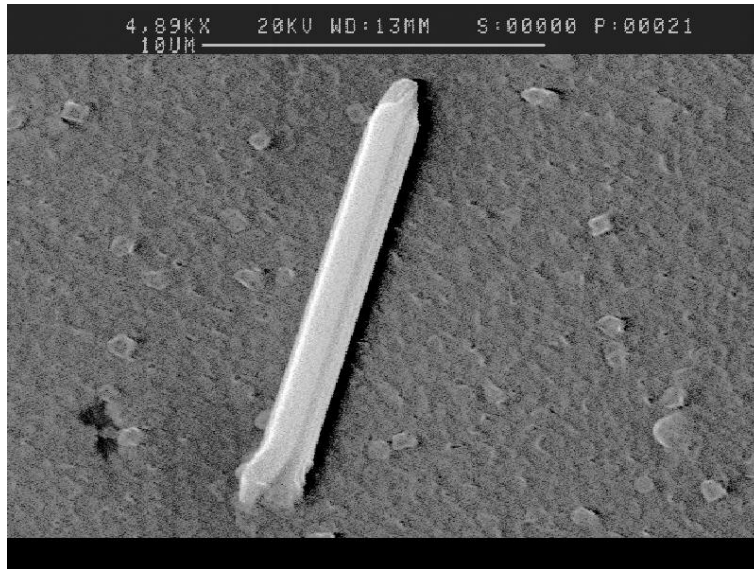
Figure 22 Whisker on the Surface of Al Film Annealed at 427°C for 2 Hours.
