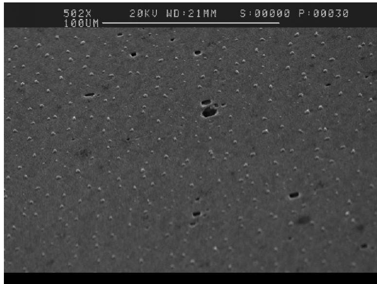
Figure 16 SEM Micrograph of Si Substrate After Annealing at 550°C for 2 Hours. Reveals the Presence of Si Precipitates and Dissolution Pits. (Al Film Removed by Etching with H 3 PO 4 )
