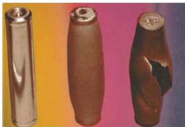
Figure 15: Irradiation Creep of Nuclear Fuel Pin Cladding [23]
