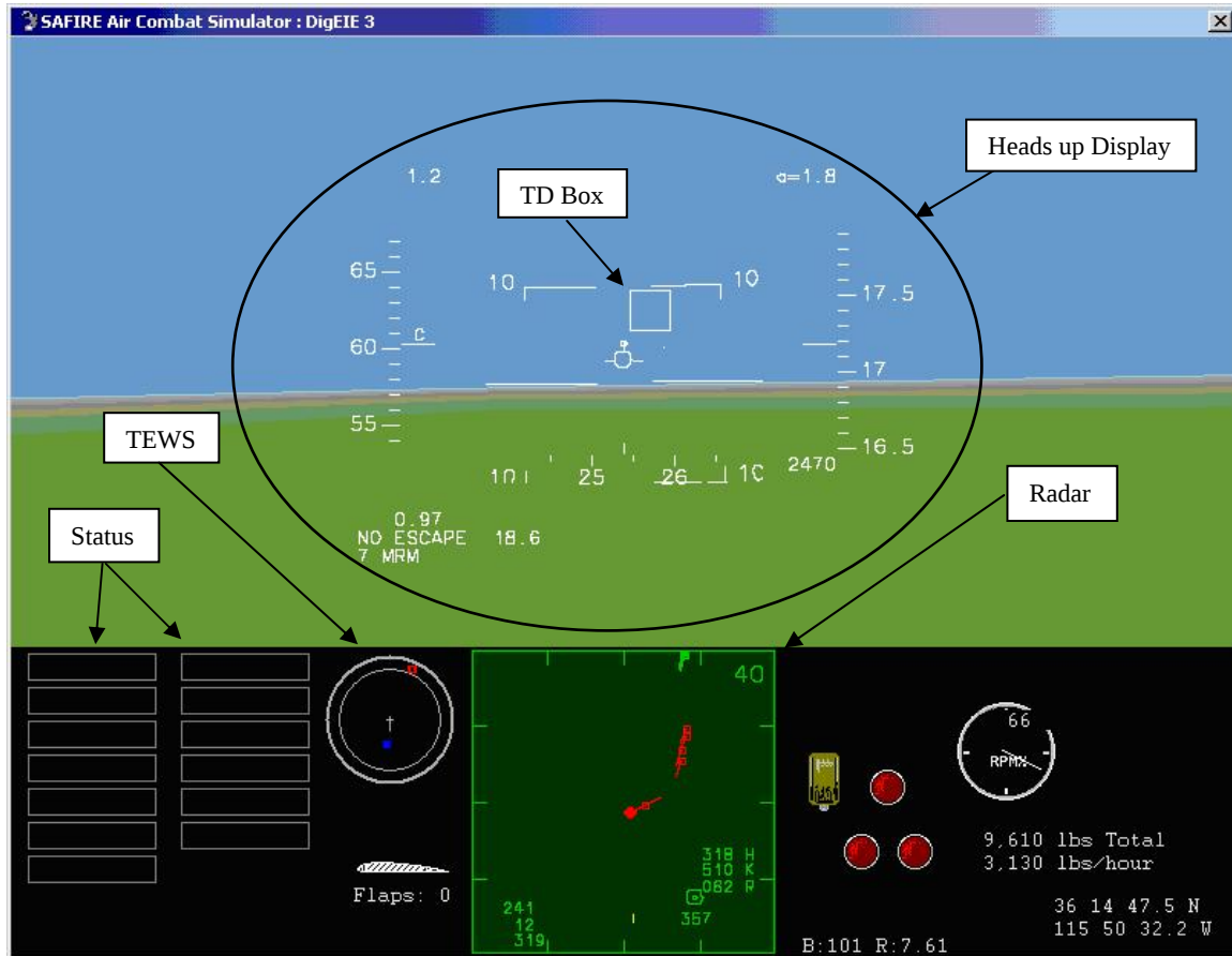
Figure 7. This is a screen capture from one of the blue fighter crew stations. The top portion of the display is the out-the-window scene with the HUD overlaid. The bottom section includes the radar display, the tactical electronic warning system (TEWS), engine, landing gear, flaps, and other status information. This screenshot was taken with the two blue aircraft in a lead-trail formation. The other blue aircraft can be seen on the TEWS display as a trailing blue dot. The red dot on the TEWS display indicates the direction of emissions from enemy aircraft.
