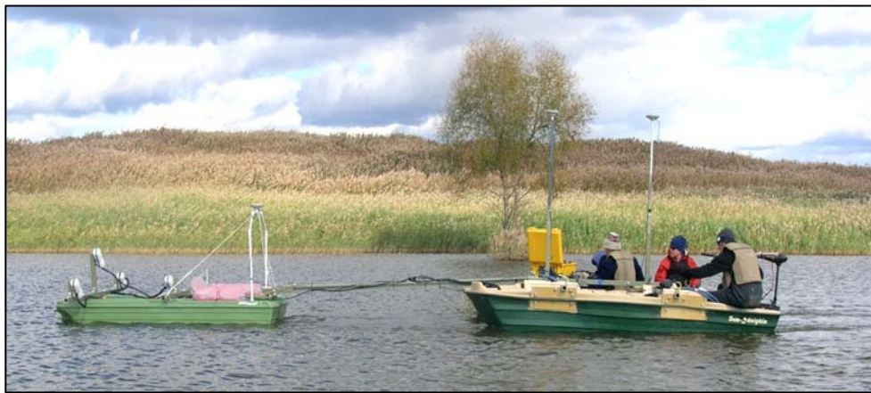
Figure 3. Tetra Tech shallow water UXO detection platform.
