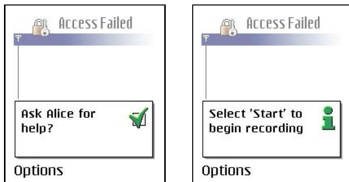
Figure 6: When a proof cannot be generated locally, the user is asked to approve a help request, which can be annotated with an audio clip.
