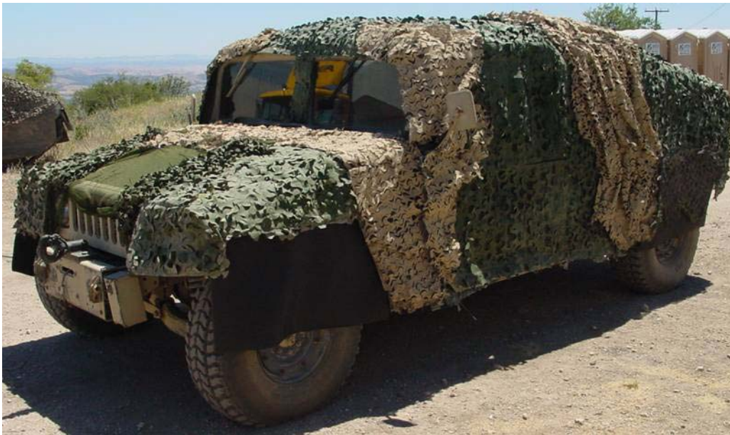
Figure 7 and 8. HMMWV with thermal insulation, camouflage netting, and conveyor belt material
