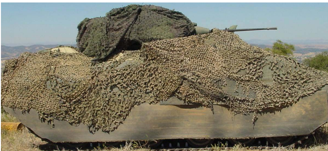
Figure 9a and 9b. M2A2 Bradley with depot level camouflage - conveyor belt over the vehicle surface augmented by a Colebrand (UK) Solar Blanket, and 2 types of US Camouflage Nets, the LCSS (Lightweight Camouflage Screen System) and ULCANS (Ultra Lightweight Camouflage Net System)
