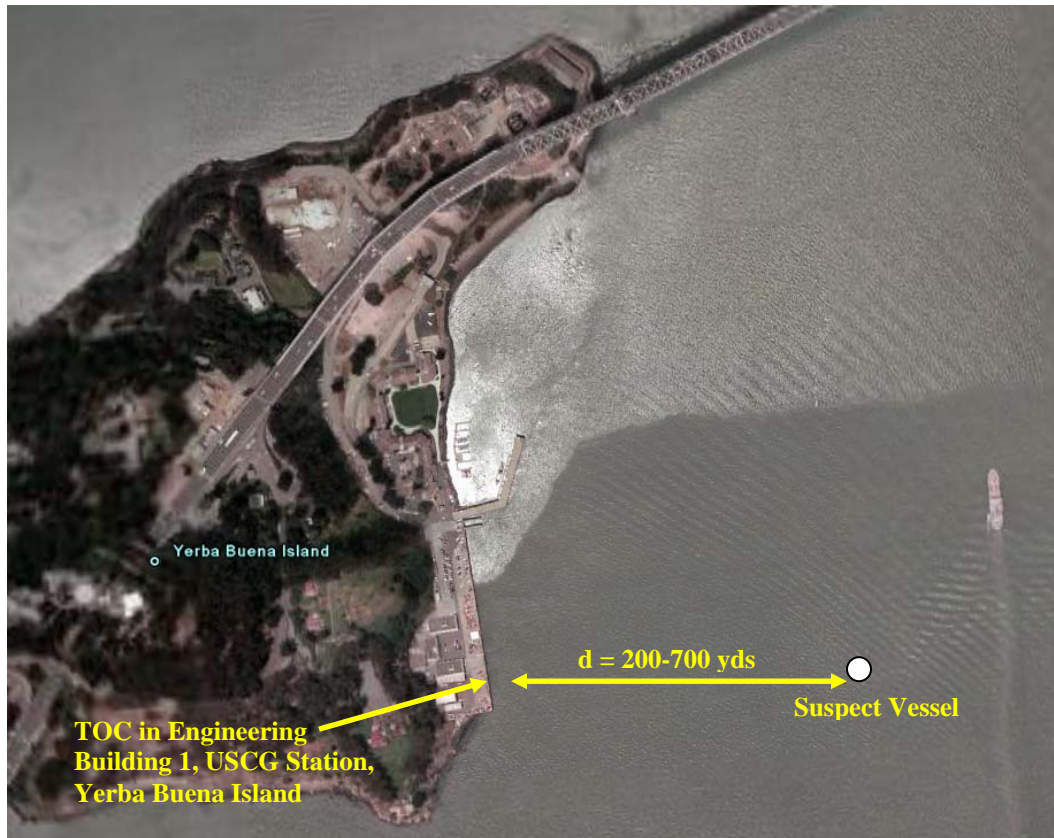
Figure 40. 802.16 Link between TOC and Suspect Vessel
