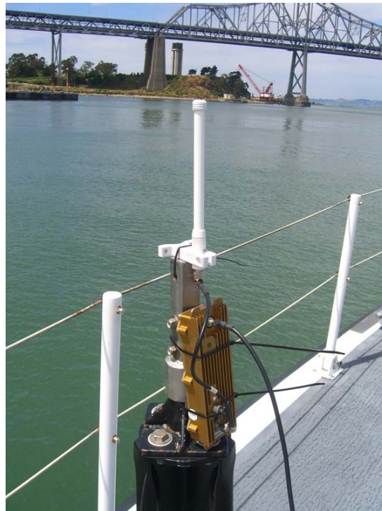
Figure 38. 6 dB omni 802.16 Antenna Onboard the Target Vessel
