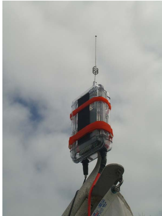
Figure 37. 900 MHz Antenna Onboard SFPD Marine Unit-3 RHIB
