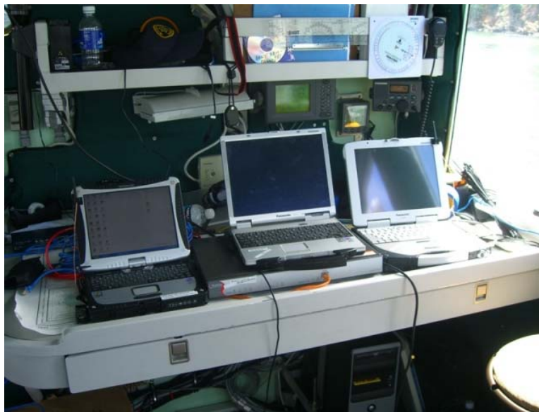
Figure 36. Suspect Vessel NOC Laptops (From Left to Right: Network Monitoring / SolarWinds, Collaboration / Groove, ITT Mesh Access Point / GPS Receiver-Poster)
