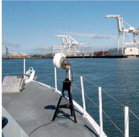
Figure 35. 802.16 Link Directional Antenna Onboard the Target Vessel (After: Bordetsky, 2006)
