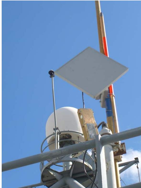
Figure 12. 802.16 Antenna Onboard the GEM STATE (GEM STATE-USCG Tern Link)
