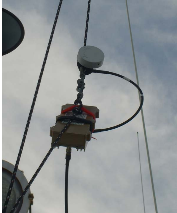
Figure 15. 802.16 Antenna Onboard the USCG Tern
