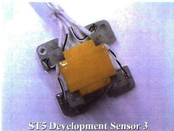
Figure 9. The 3-axis ring-core fluxgate sensor fabricated by UCLA for ST5. A similar design will be used for DSX. The DSX sensor will occupy a volume of 5x5x5 cm.
