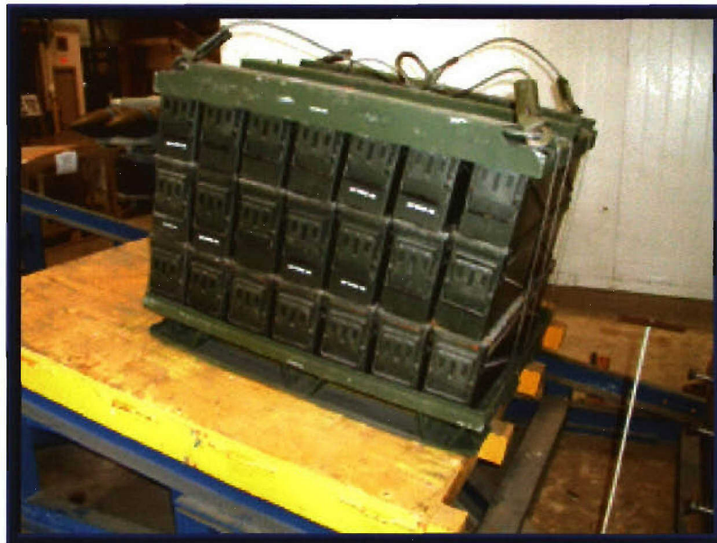
Photo 9. Incline-Impact Testing of the Test Unit.
