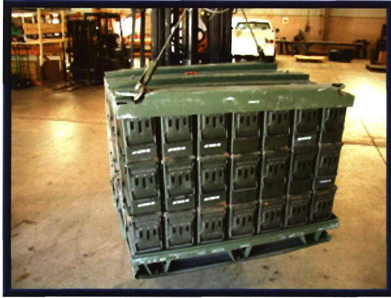
Photo 10. Two-Point Sling Compatibility Testing of the Test Unit.
