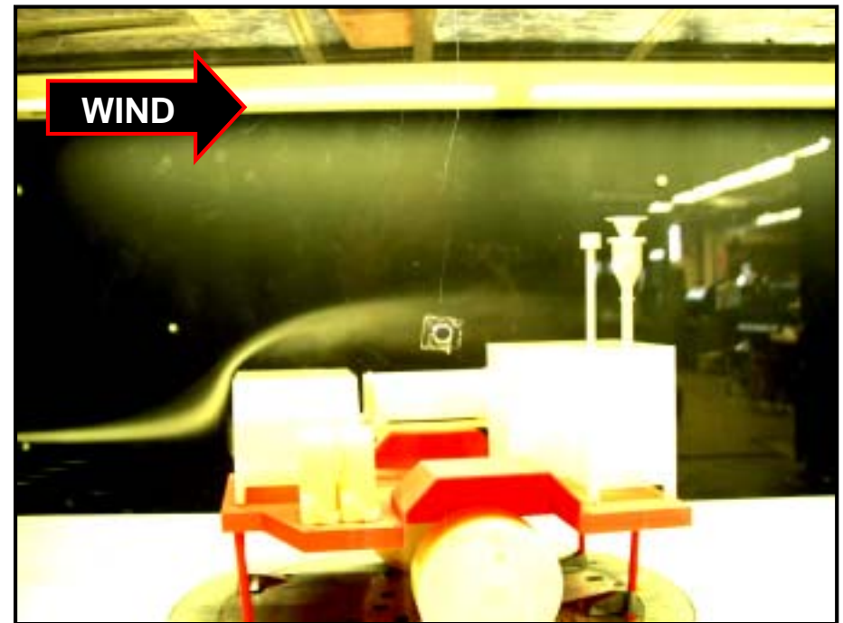
Trailer forward into wind orientation
