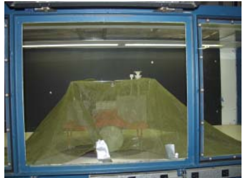
Trailer draped in one layer of fine weave netting
