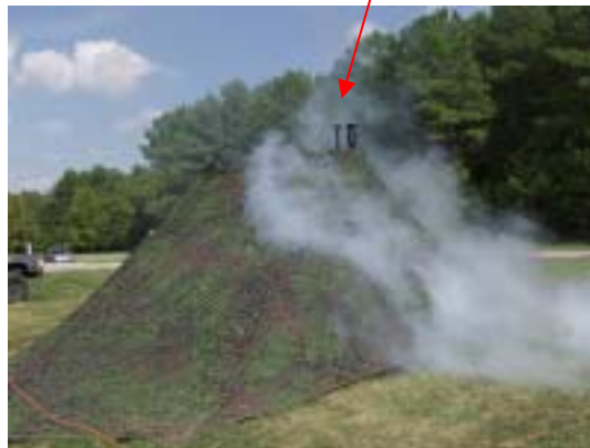
Flow going over vehicle and netting to inlets
