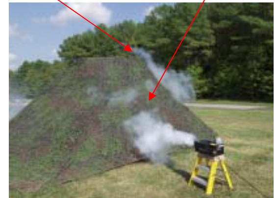
Flow going through netting and emerging/persisting in rear wake area
