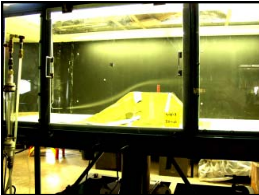
Flow from 3.5-ft approach level is directed over inlet
