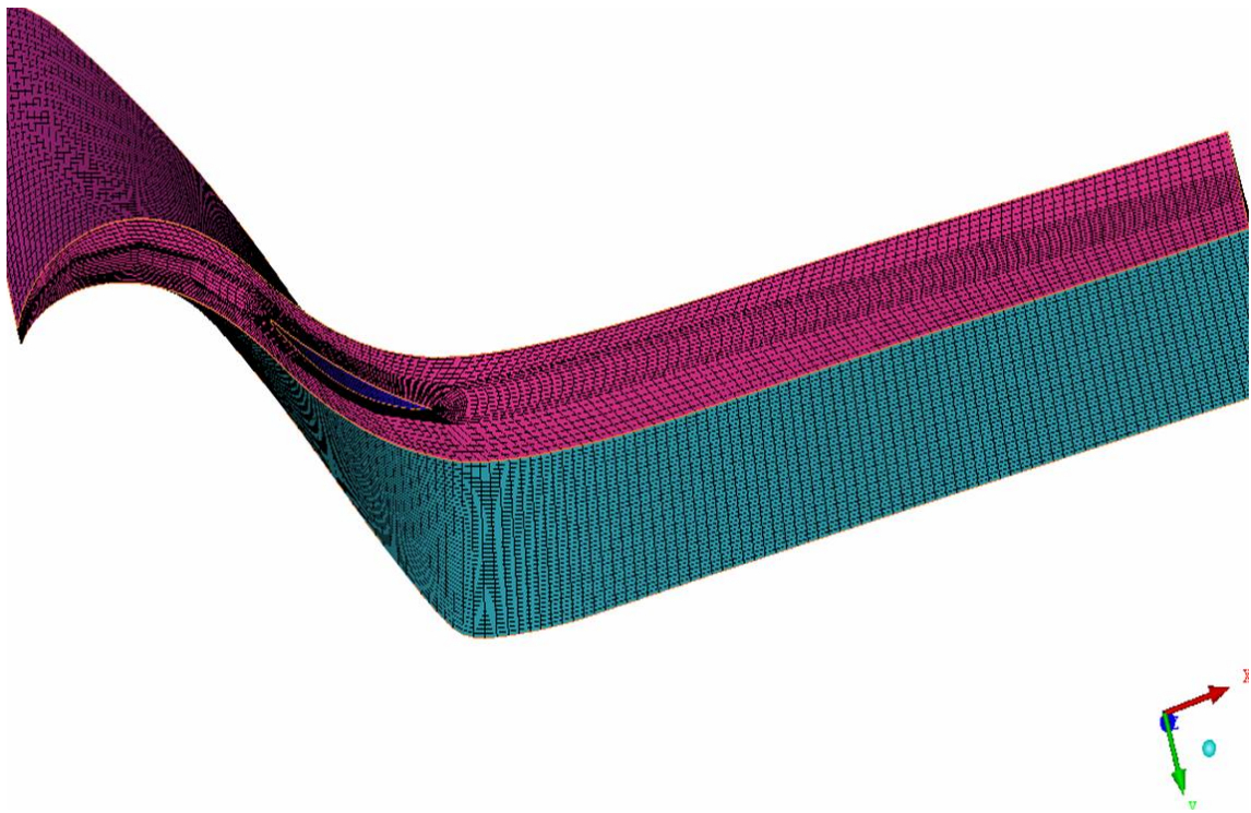
Figure 16. Shroud Mesh Created in ICEM-CFD
