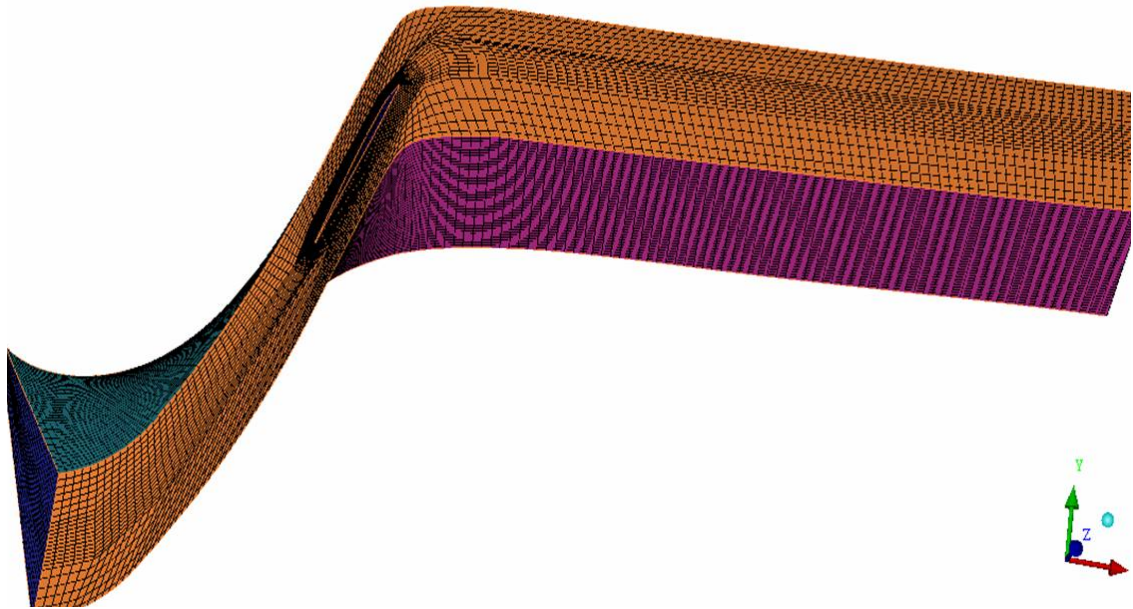
Figure 15. Hub Assembly Mesh Created in ICEM-CFD
