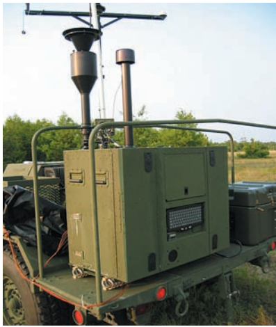
Joint Biological Point Detection System Trailer Variant at Multi-Service Operational Test and Evaluation.
