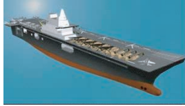
A. Large ship for aviation, weapons, and support. Displacement: 57,000 tons Length: 250 m
