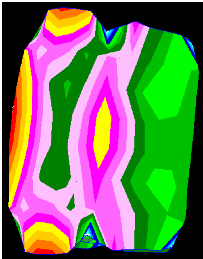
Figure 41. Deformation of 7.47 \times 10^{-3} m (FAILURE) in Satellite Side Panels (Thickness 0.007 m, Applied Heat Flux 1000 \text{ W/m}^2 )
