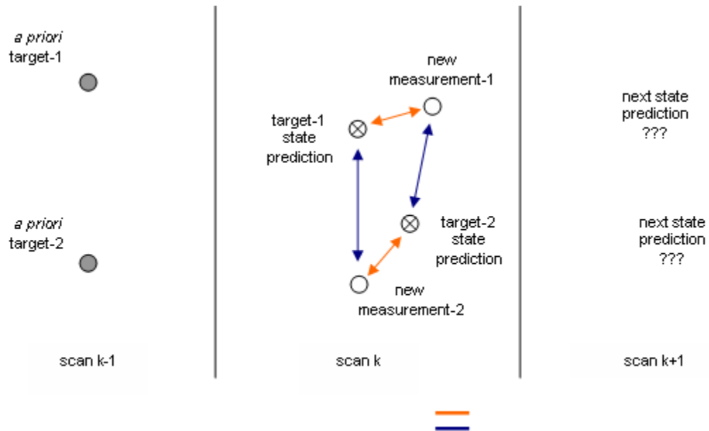
Figure 19. Multiple-target tracking (2-D) scenario. An illustration of the difficulty in correctly pairing new measurements with their state prediction so subsequent predictions converge on the true track.
