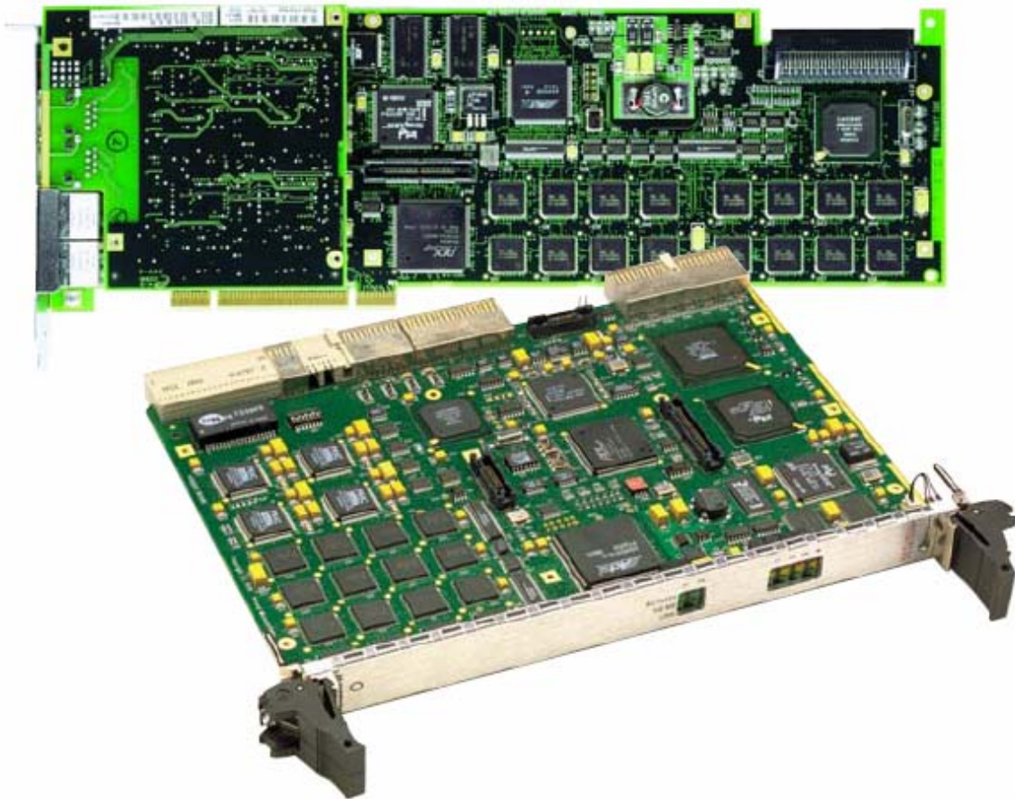
Figure 13. Natural Microsystems CG 6000 Telephony Board [From Ref. 8]
