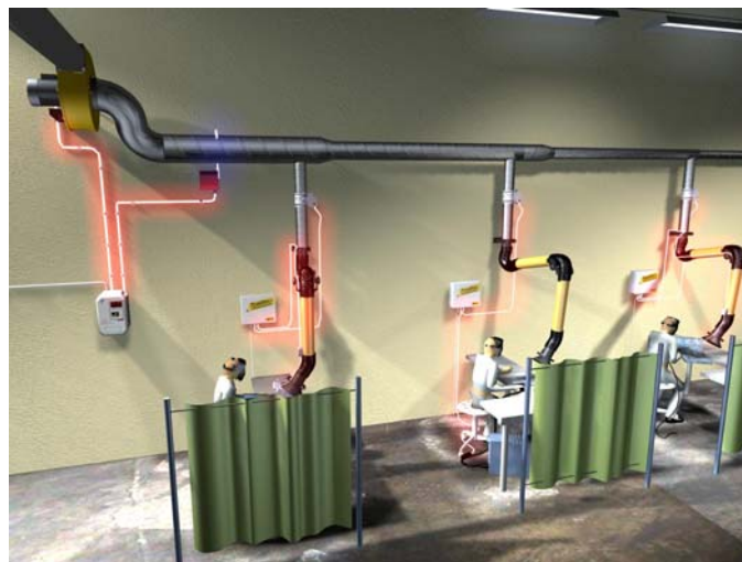
Figure 56. Schematic of a welding shop demand based local exhaust system.
