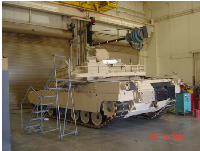
Figure 34. Example of vehicle exhausts at maintenance shop for A1M1 tanks.
