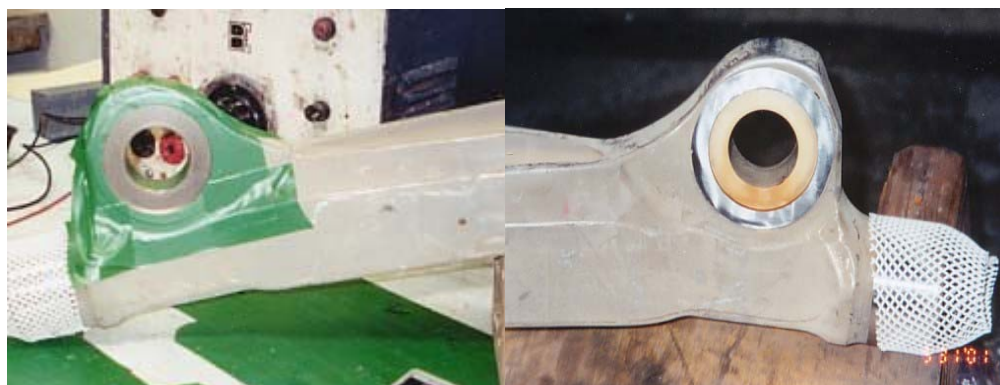
Figure 50. Part masking (before and after plating).
