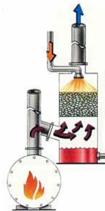
Figure 17. Cut-away view of a boiler stack economizer.
