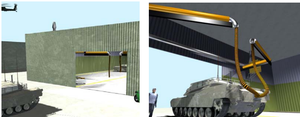
Figure B9. Boom-based exhaust system allows to capture exhaust fumes from a M1A1 tank moving into and out of the maintenance bay.
