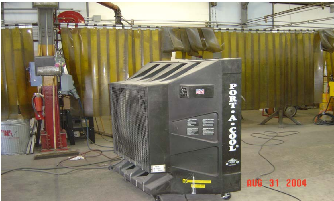
Figure 11. Roll-around evaporative cooler now in use at Sierra Army Depot.
