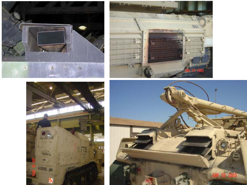
Figure 36. Examples of tail pipes and exhaust grills of typically serviced military tactical equipment.
