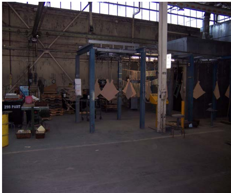
Figure 40. Paint booth with attached oven.
