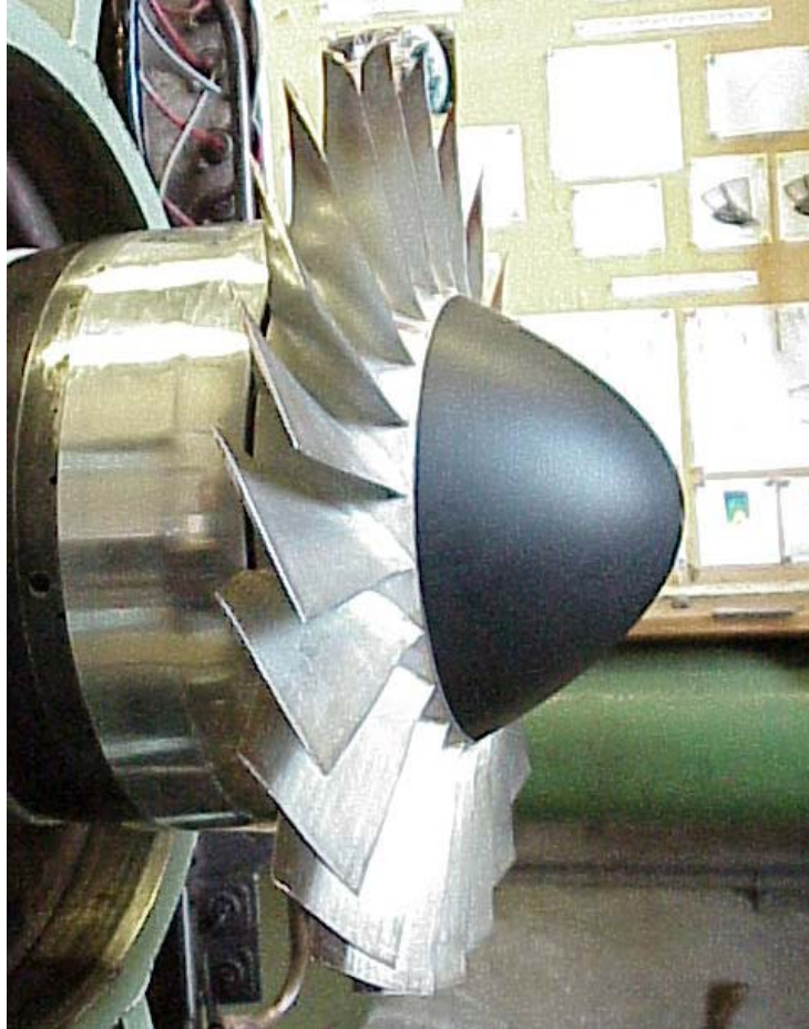
Figure 2. Rotor-only configuration of the transonic compressor rig (From Ref. 8)
