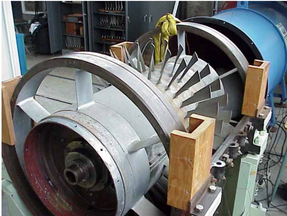
Figure A4. Top shell removed/blocks in place to guide rotor out of bottom shell
