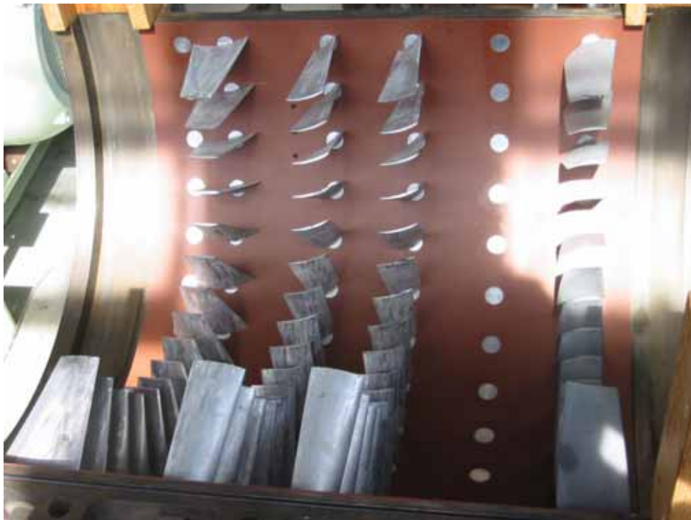
Figure A18. Bottom shell with rough-cast blades: Inlet guide vanes (far right), stator blades (middle two rows), exit guide vanes (far left)
