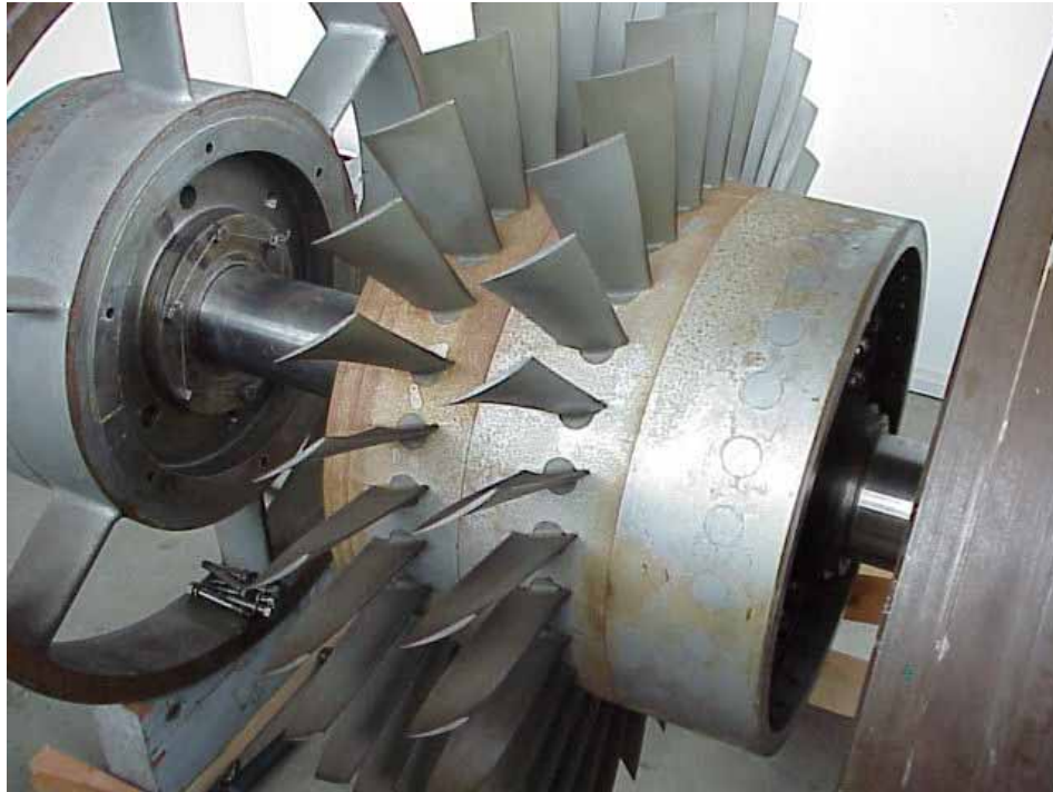
Figure A6. Close-up of smooth-cast (plastic) rotor blades and rotor hub
