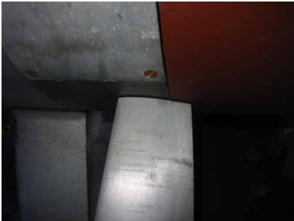
Figure A24. Inlet guide vane clearance with hub
