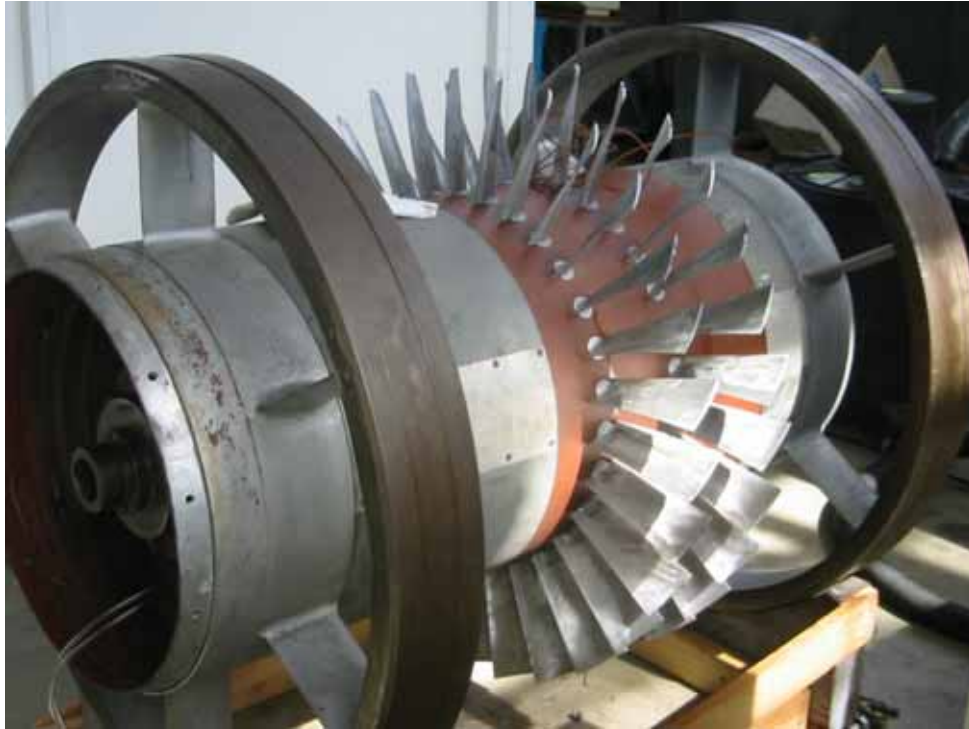
Figure A19. Rotor hub completely assembled with rough-cast blades
