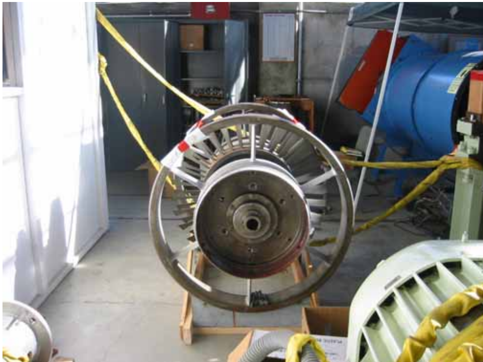
Figure A5. Rotor hub on blocks
