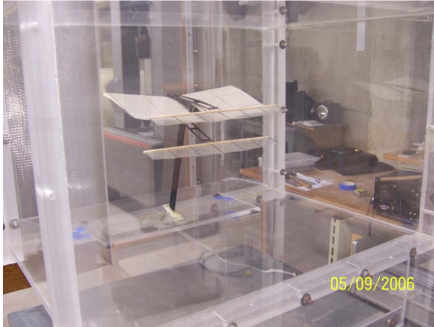
Figure 35. Complete Horizontal Model in the Test Section
