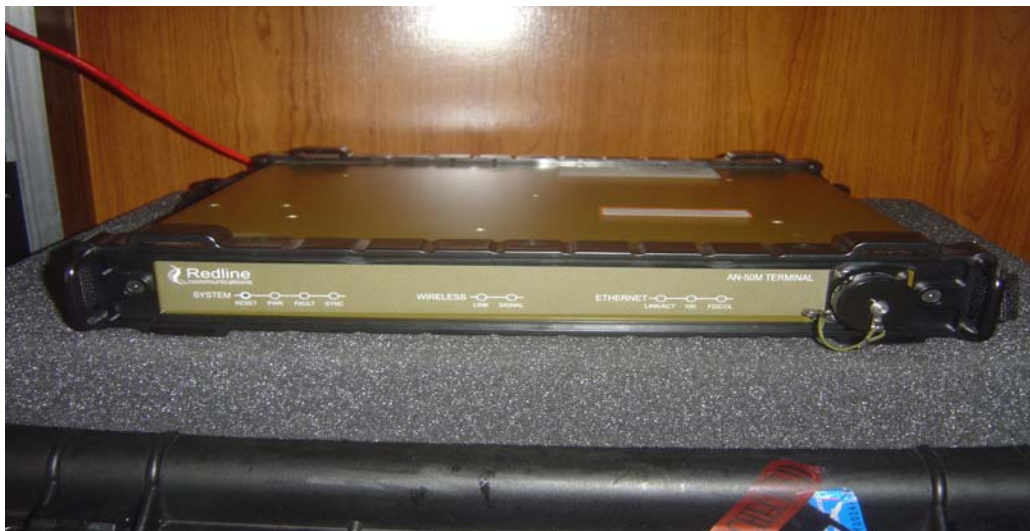
Figure 24. AN-50M Wireless Base Station
